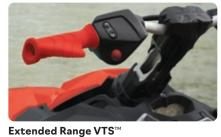
(Variable Trim System) Offers double the range of the regular  $VTS^{\mbox{\scriptsize M}}$ for greater ease when executing tricks.
