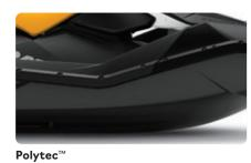
Innovative material that reduces weight while optimizing performance and efficiency. The color-in molding is more scratch-resistant than fiberglass.
